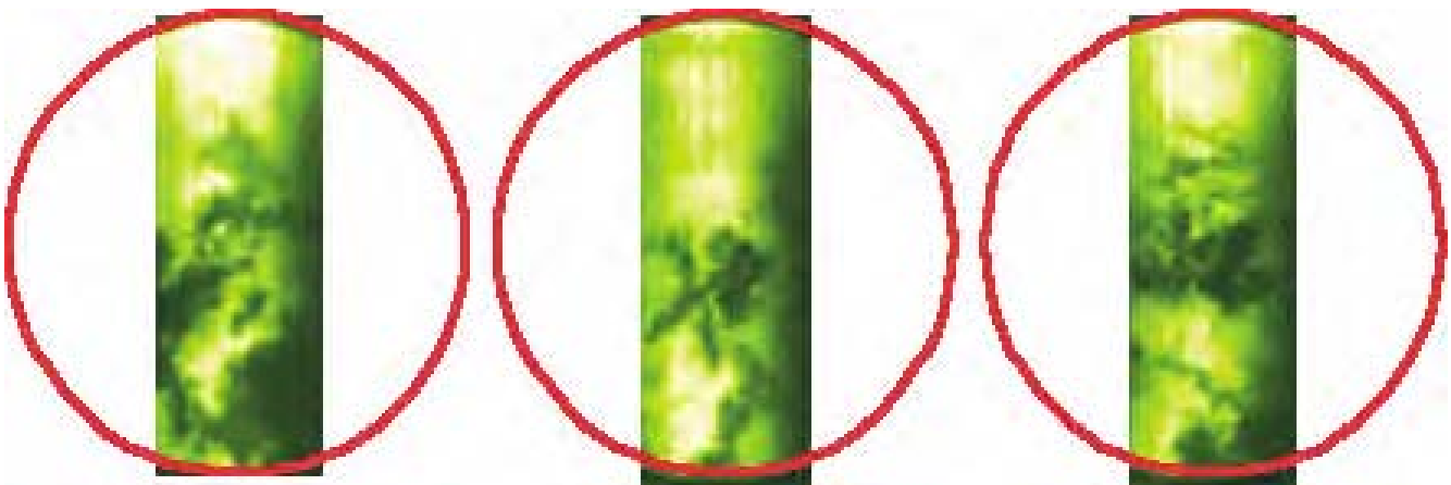
Visualization of fuel concentration by laser-induced fluorescence in a gasoline CAI engine - the dark zones correspond to burned gases (4 deg. CA ATDC - 1500 rpm – lambda 1.12 – CR=10)
