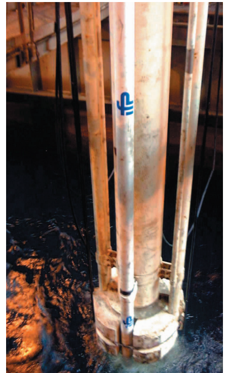
Field test of an hybrid line on the Pride Angola drillship.
