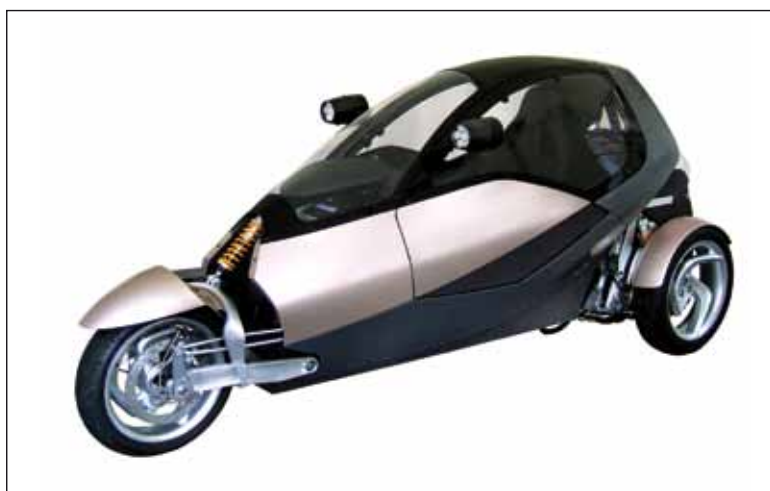
Clever vehicle with tilting cabin in curve.
