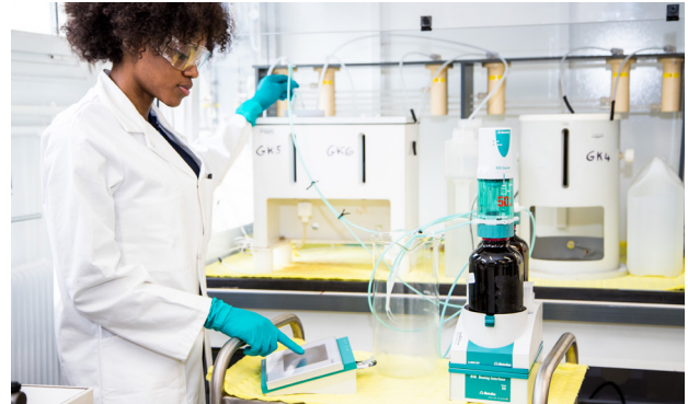
Organic matter isolation system (IFPEN kérogénatron®) 8 small and 3 big reactors - Automated dosimeter for acids
