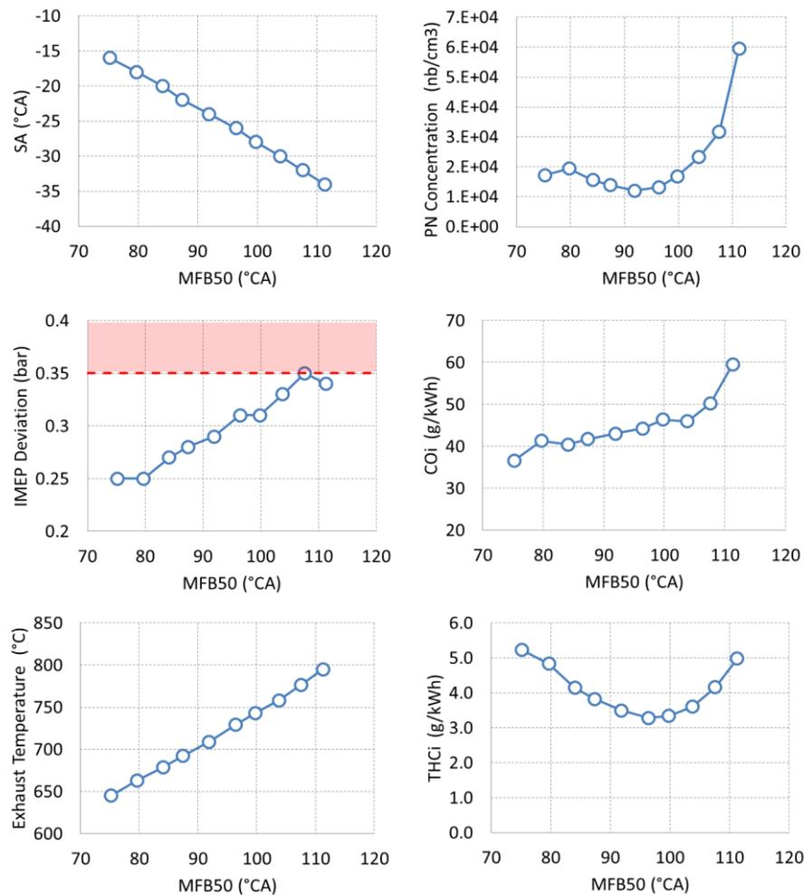
Fig. 9: Spark advance sweep on 1350rpm/1.7bar IMEP operating point ( $T_{water}=T_{oil}=40^{\circ}C$ ).
