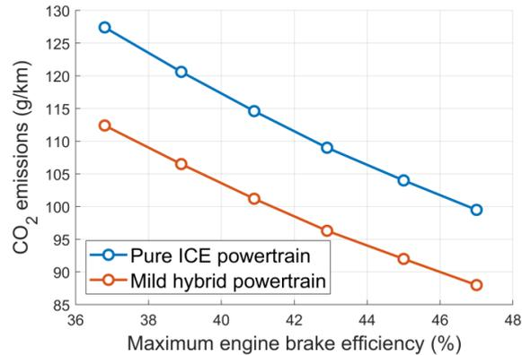
Fig. 1: Impact of engine efficiency on CO<sub>2</sub> emissions of thermal and mild hybrid vehicles.
