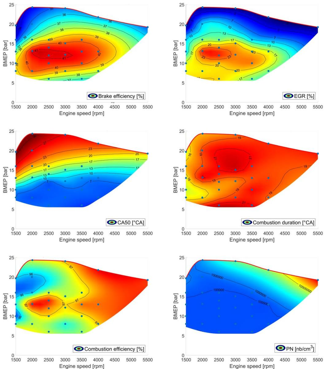
Fig. 7: Experimental results obtained at test bench.
