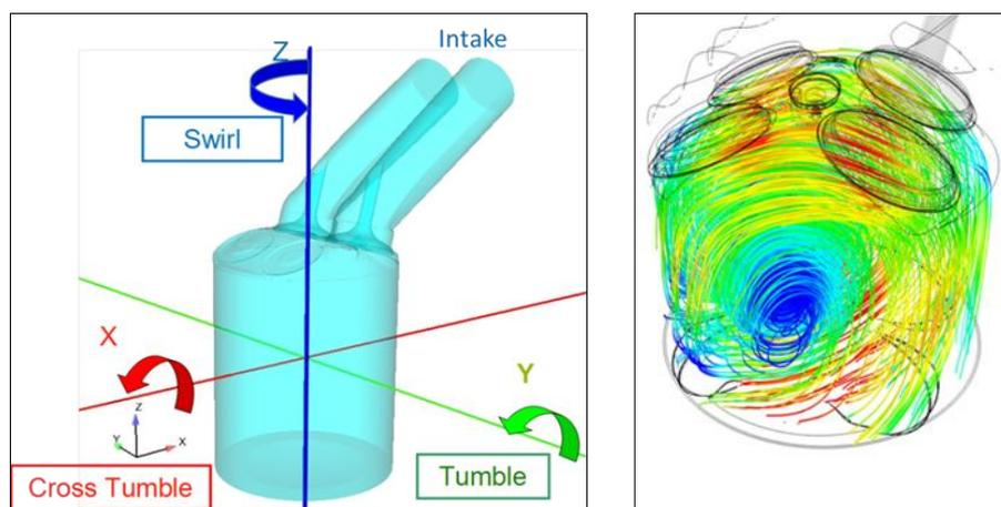
Fig. 2: Swumble™ fluid motion [4] is a combination of Tumble and Swirl motions.
