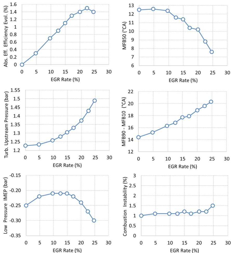
Fig. 10: EGR rate sweep on 3000rpm/12bar BMEP operating point.
