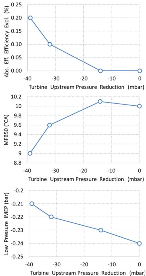
Fig. 11: Impact of turbine upstream pressure reduction on a 3000rpm/12bar BMEP operating point at the same EGR rate (20%)
