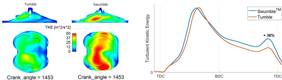
Fig. 3: Turbulent Kinetic Energy distribution obtained and flame fronts on both Tumble and Swumble engines.
