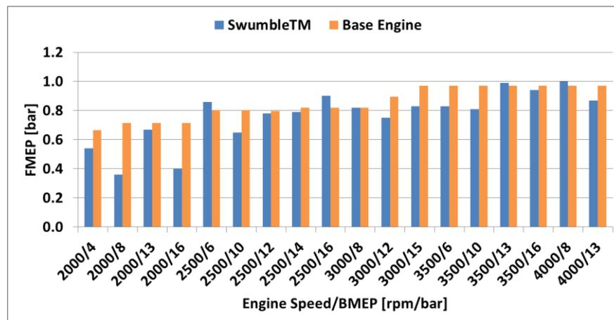
Fig. 6: Friction mean effective pressure: comparison with base engine level.
